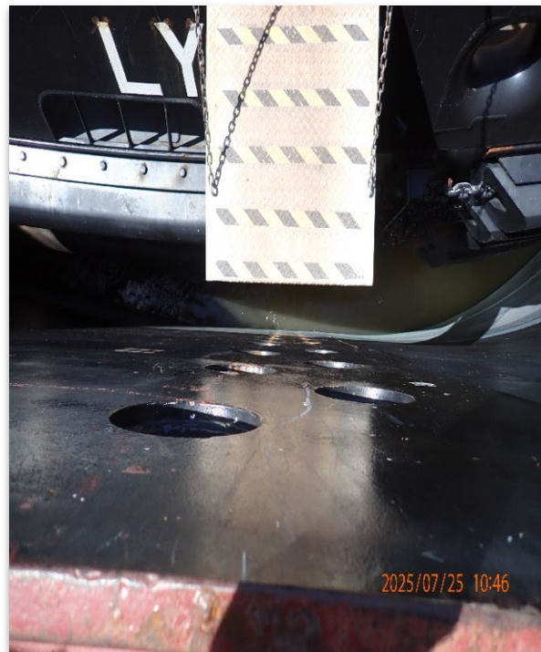
Figure 2: View from the deck of the barge showing the pigeonhole vertical drop to the tow notch
