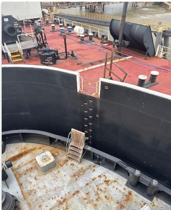
Figure 1: Barge pigeonhole embarkation station
